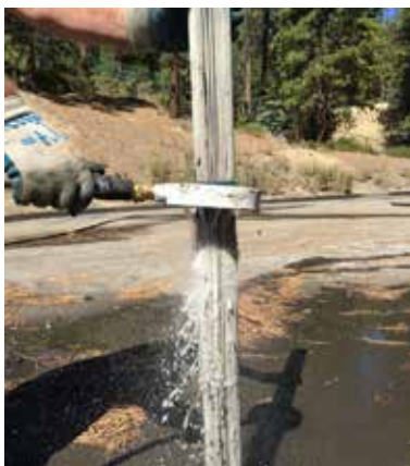
The Jellyfish Filter tentacle is light and easy to clean
